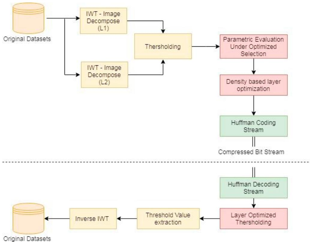
Fig. 1. System Architecture for Image compression using Machine learned pixel clustering approach
